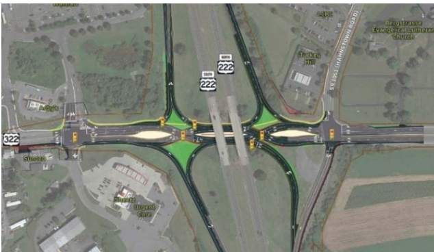
Reconfiguring the interchange to a DDI was determined to be the best approach to meet the project’s goals achieving a benefit to cost ratio of 13:1 and subsequently advancing to final design.
